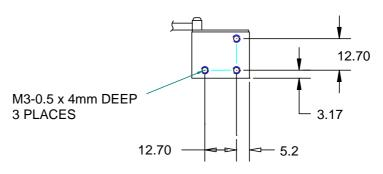
Ensure adequate heaksinking through mounting surface, especially at higher RF powers.
