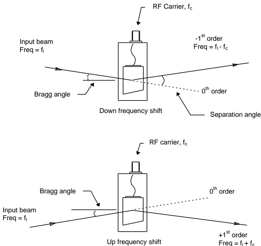
Maximum diffraction efficiency into the first order is achieved when the input light beam to the AO device is aligned at the Bragg angle and the RF power is adjusted for saturation.
