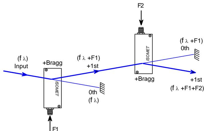
Alternatively a multiple pass can be made through a single AO device using (say) a retro reflector. The suitability of this method will depend on the beam size relative to the maximum useable crystal aperture. The diagram below shows a basic double downshift configuration.
