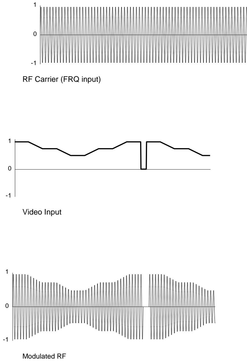
Figure 3, Typical Amplitude Modulation Waveforms
