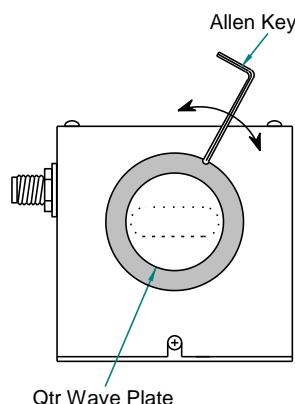
NOTE. For the **LS110 XY**, the waveplates are secured with locking screws. Remove cover to gain access.
