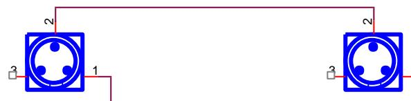
The interlock signal must be connected. Contacts closed for normal operation.
