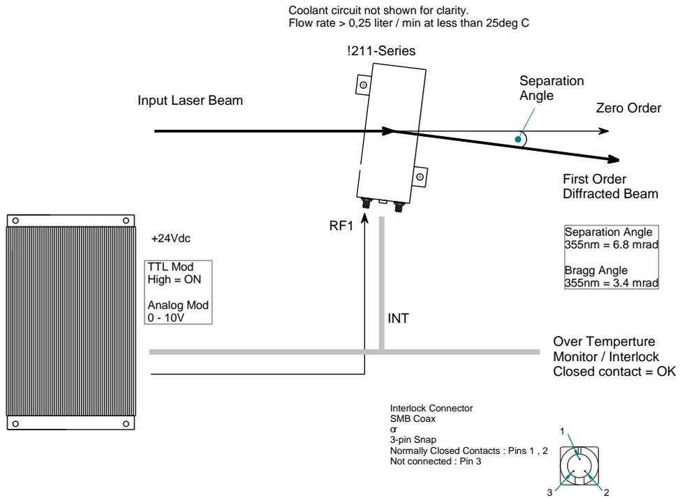
Figure 4: Typical Connection Configuration
