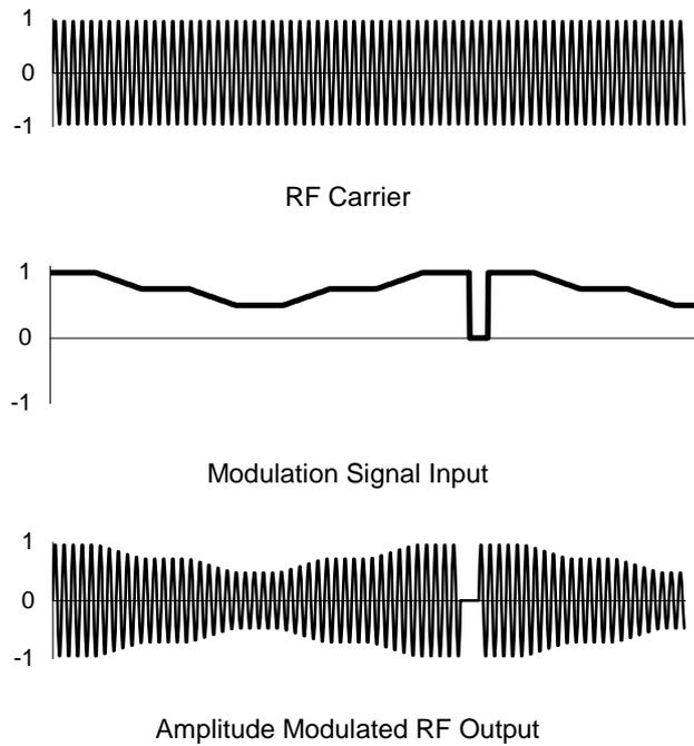
Typical analog modulation RF waveforms are shown above. For the RFA910 and similar drivers, the modulation input is a combination of analog and digital control as illustrated below.
