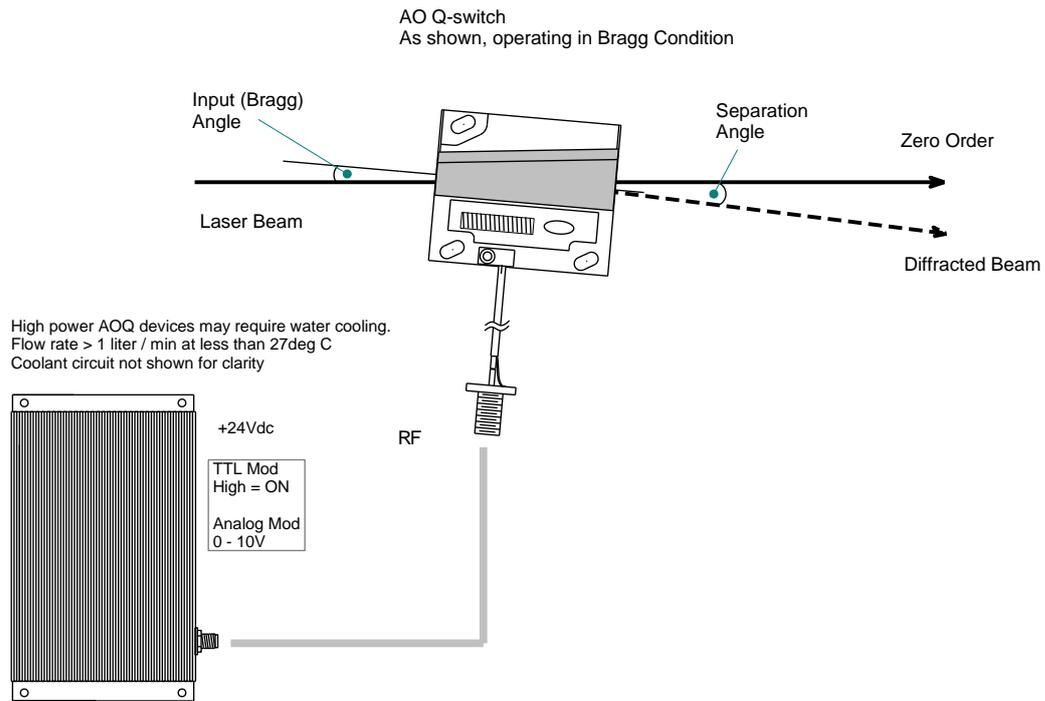
Figure 4: Typical Connection Configuration
