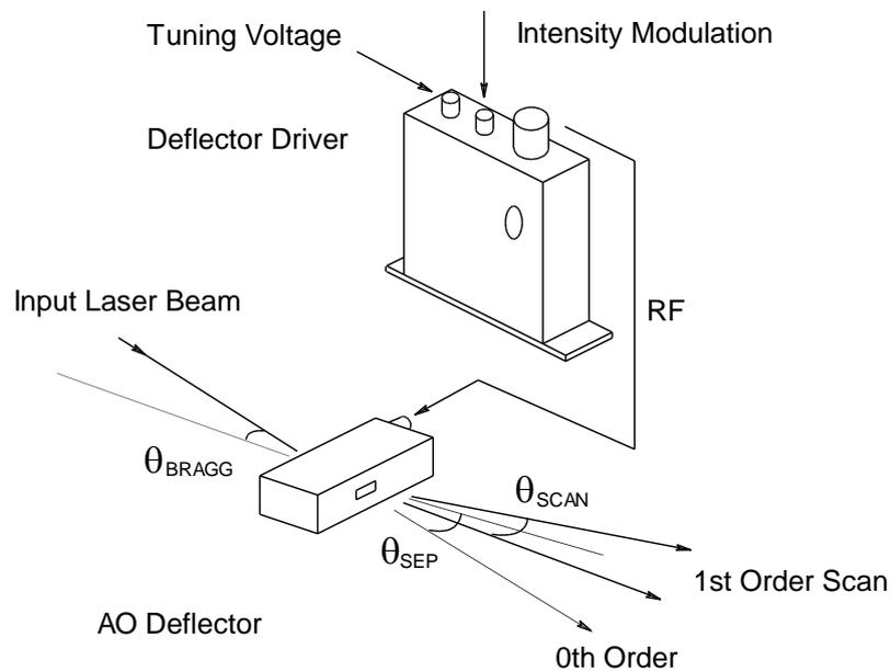
The input Bragg angle, relative to a normal to the optical surface and in the plane of deflection is given by:
