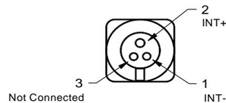
The interlock connection becomes open circuit disabling the RF output, if the temperature of the modulator exceeds 32°C or the internal driver temperature exceeds 43°C. An LED indicator illuminates when the Interlocks are closed and the RF is enabled. An opto-isolated interlock status signal is available across pins 2 and 7 of the D-type. The opto is low impedance when interlocks are valid.
