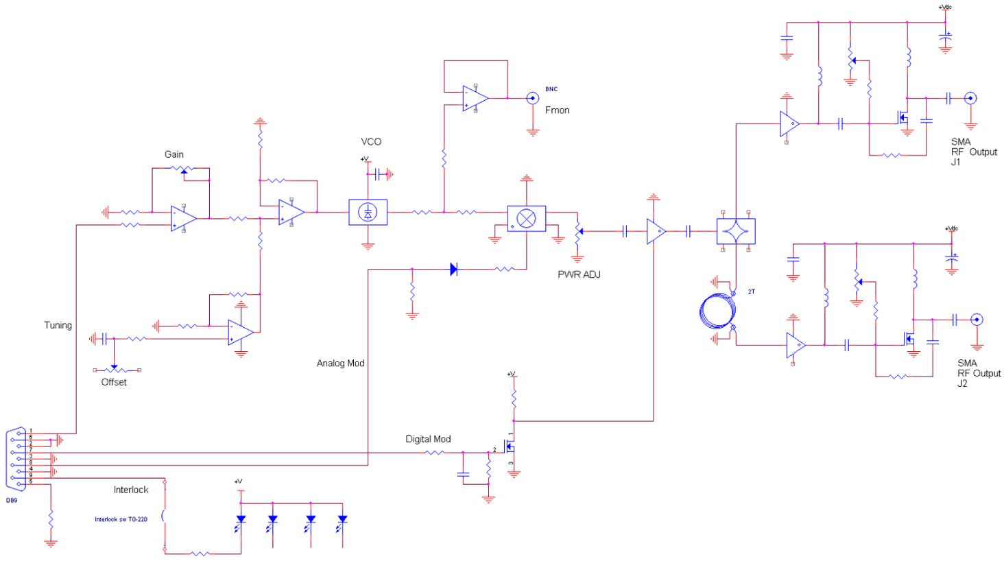
Figure 2, Driver Block Diagram
