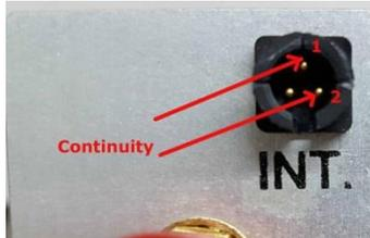
For Germanium and some Quartz AO devices the typical over-temperature threshold is 32degC. The switching hysteresis is 7-10deg C. Therefore, it is necessary to reduce the coolant temperature to below 18degC to reset the thermal switches. (closed circuit)
