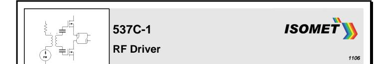
The 537C-1 is an analog modulation driver designed to operate with Isomet 350MHz AO modulators for high speed control of laser beam intensity.
